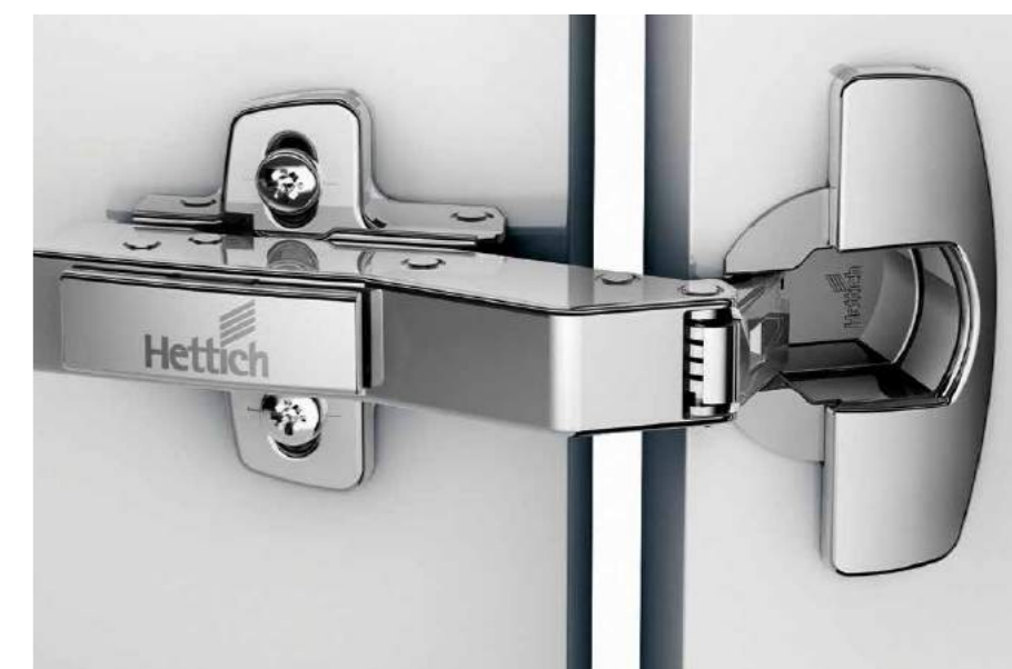
W30 full overlay angle hinge (opening angle 95°, for 30° face angle)
