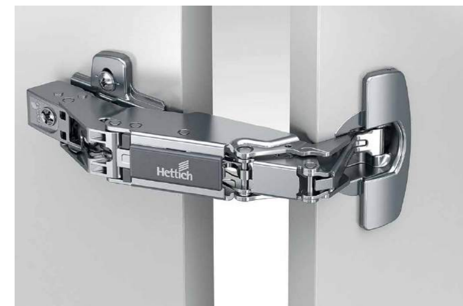
Full overlay wide-angle hinge in Internat Design (opening angle 165°, for 90° construction)
