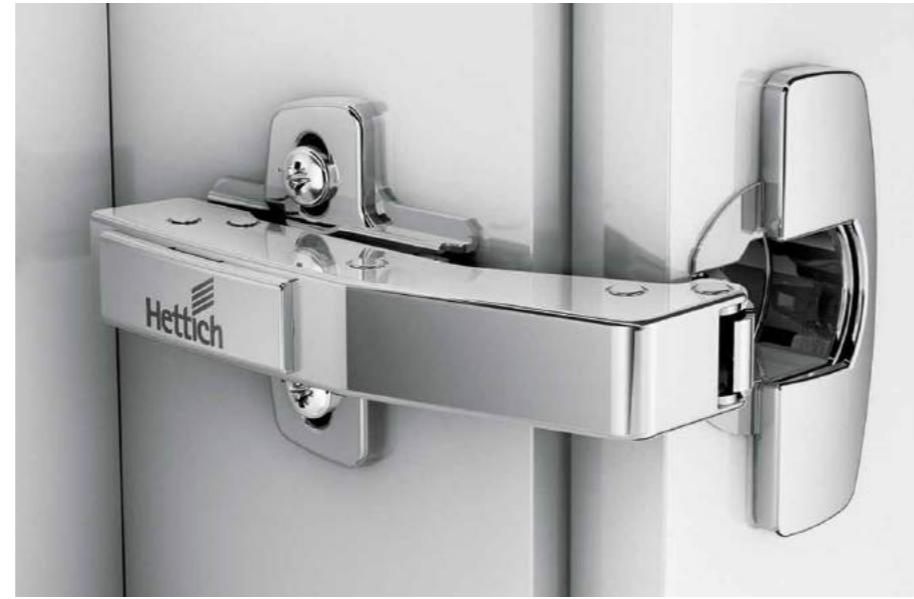
W90 blind corner inset hinge (opening angle 95°, for 90° face angle)
