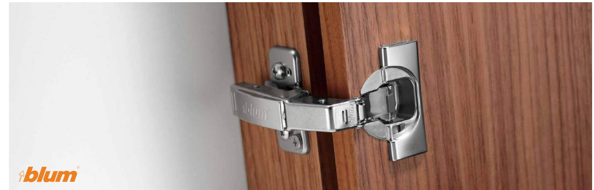
Blind corner overlay hinge with integrated BLUMOTION (opening angle 95°, for 90° face angle)
