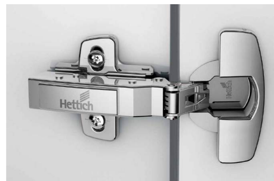
Standard hinge full overlay / half overlay / inset (opening angle 110°, for 90° construction)
